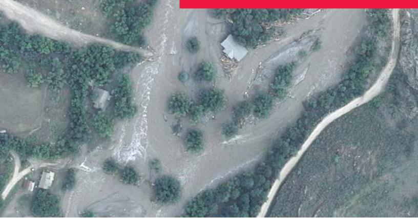
The resolution in the color images from the DMC camera was good enough to pick out whitewater plumes and turbulence in the Poudre River, especially where the water had overflowed its banks.
